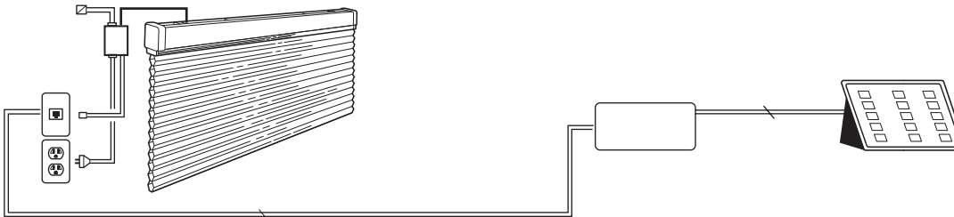
I. Automation Control System with Infrared (or Radio Frequency) Remote Control
