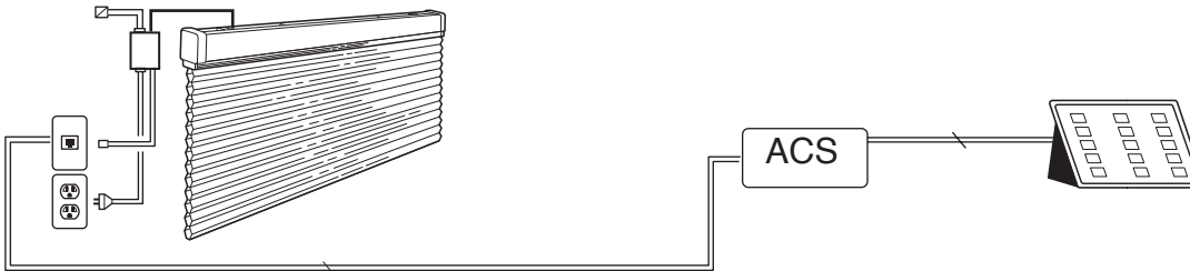
G. Automation Control System with Radio Frequency Remote Control
