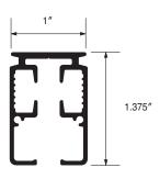
Recommend installation of brackets in intervals of 30".
